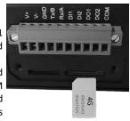
When inserting a SIM card, ensure the SIM card has the correct orientation. Do NOT insert the SIM card at an angle or use force. There is also an SD card slot next to the SIM card slot, the use of this is not currently supported by the firmware.
