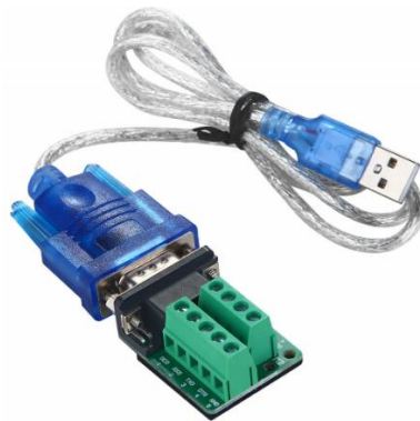
Figure 4: RS232 to USB adaptor
