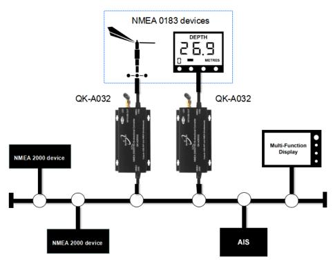
Figure 1: Example setup
