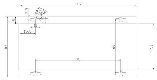
Tolerance: ±0.25 Figure 2: A032 Dimension in mm
