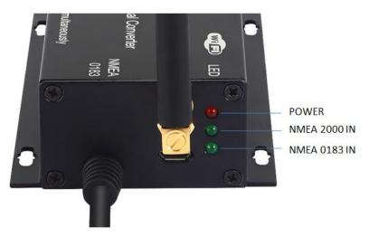
Figure 4: LED functions
