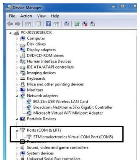
Figure 5: View of COM port in Device Manager
