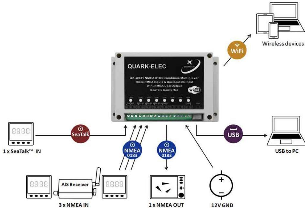
Figure 2: Typical system connection
