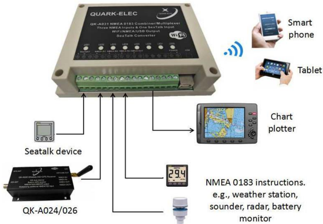
Figure 3 Operating in Ad-hoc mode
