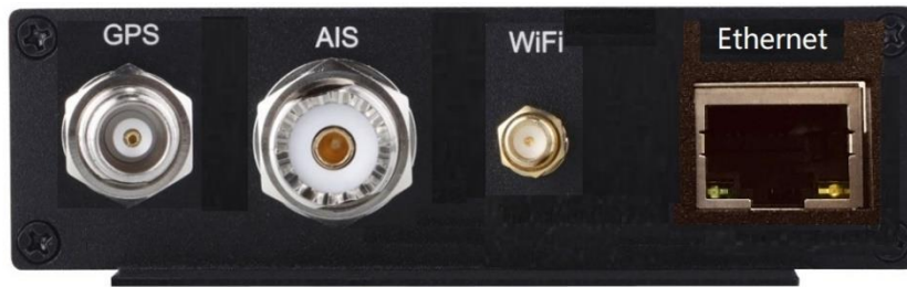
Figure 7: GPS (TNC), AIS (SO239), WiFi (SMA) antenna connections
