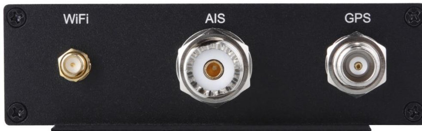
Figure 8: AIS (SO239), GPS (TNC), and WiFi(SMA) antenna connections
