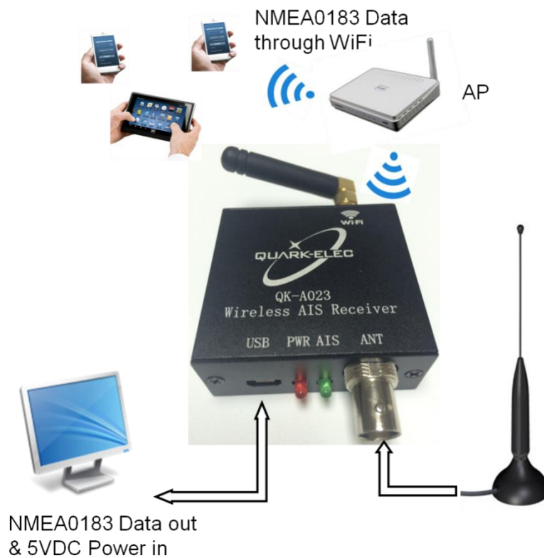
Figure 2 Typical application(station mode)
