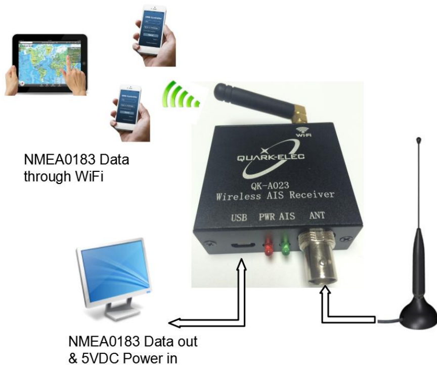
Figure 1 Typical application(Ad-hoc mode)
