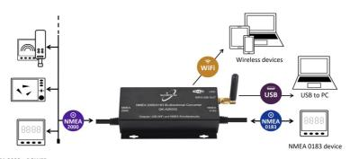
NMEA 2000 + POWER (networked input sensors, and output devices)
