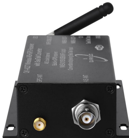
Figure 5 GPS and AIS antenna connector
