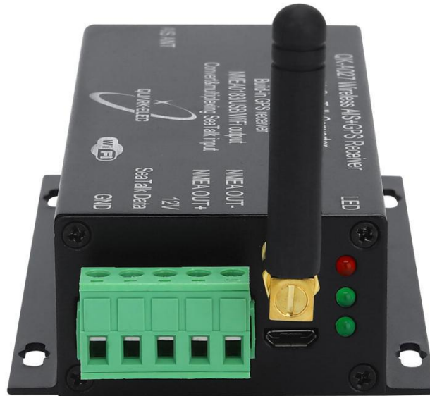
Figure 4 SeaTalk and NMEA output connector
